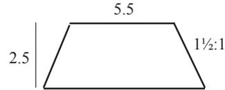
$$\begin{aligned} \text{Volume of earth work } V &= (bd+nd^2)L \\ &= (5.5 \times 2.5 + 1.5 \times 2.5^2)12 \\ &= 77.5\text{m}^3 \end{aligned}$$
